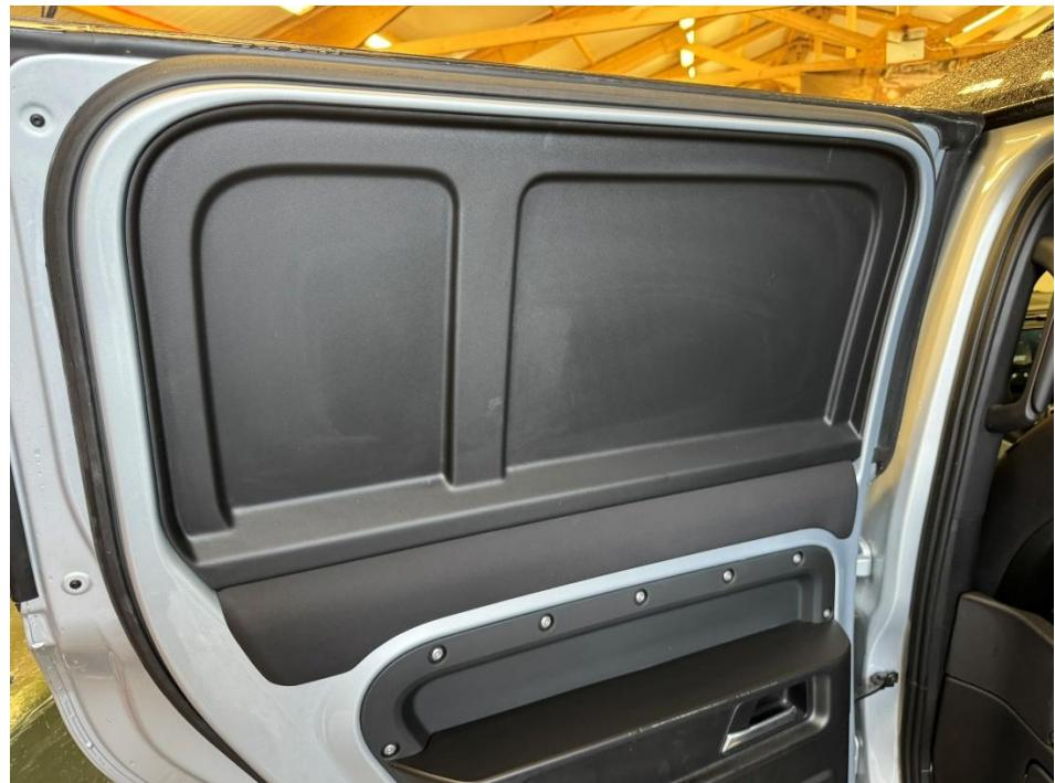
The factory window trims are attached to the window frame with a thick bead of Sikaflex adhesive in the areas marked in Red and a single strip of double-sided 3M adhesive tape marked in Green.
