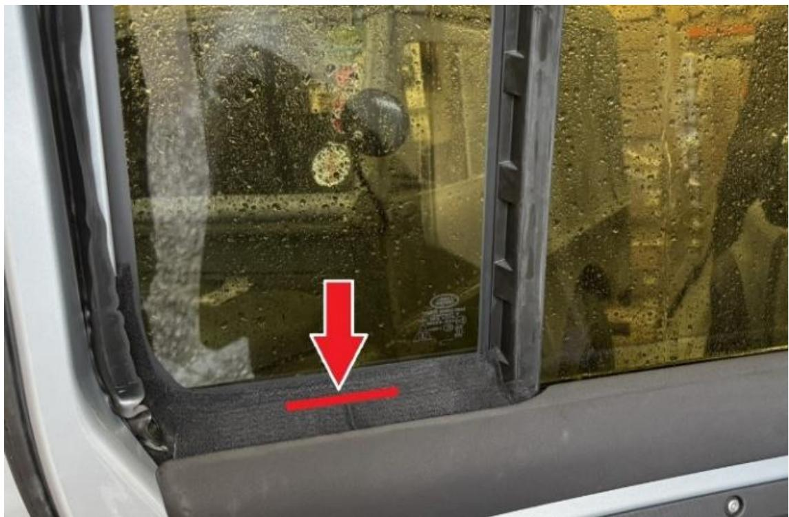
Make sure you remove the adhesive far enough beyond the vertical upright to provide sufficient clearance for the top of the plastic trim to wrap around the vertical upright in the area arrowed in red.
